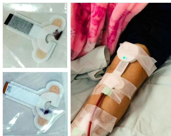
Figure 9. An example of the micro-leakage chart in the clinical trial. A tiny amount of blood infiltrated into a small area emphasized in a direction. The multi-ring design is better than a multiple point-type design for the estimation of leaked blood volume.
