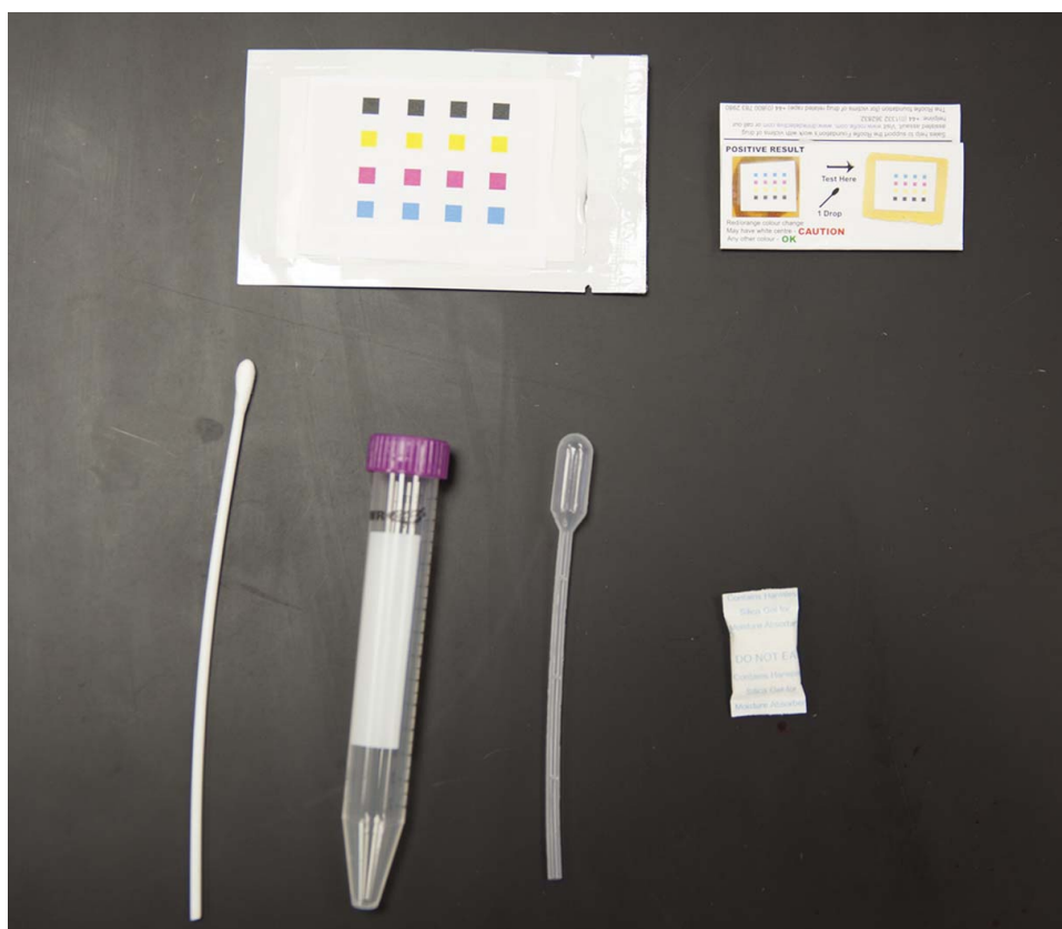
Figure 11. Prototype printed colorimetric array analysis kit. The kit contains the sensor array, disposable pipette, instructions, and silica gel desiccant sealed inside a protective foil packet.
