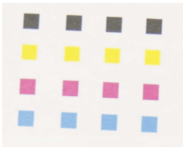
Figure 4. A colorimetric array printed with a commercially available inkjet printer showing four rows of four different sensors.
