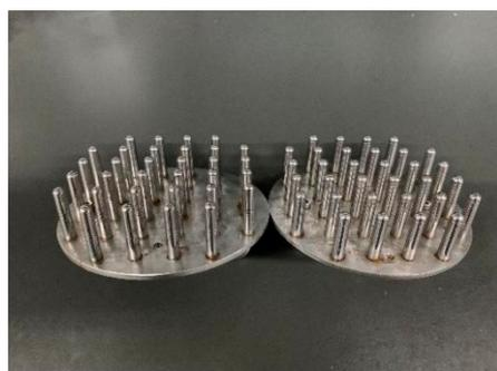
**Figure 1.** Stainless steel mold pins of capsules (cylindrical: cap,  $6.8 \pm 0.02$  mm; body,  $6.4 \pm 0.02$  mm).
