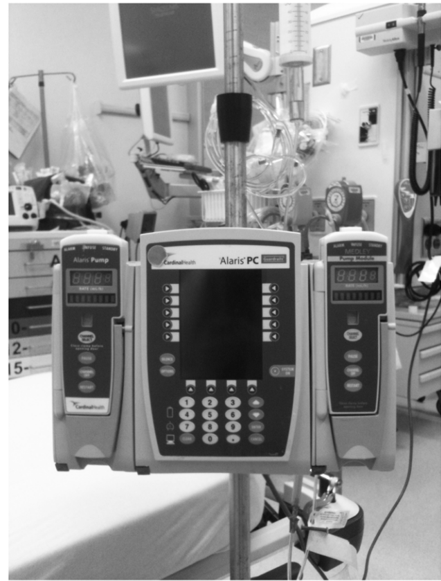
Figure 1. Regular Infusion Pump. Typical bedside infusion pump used for the administration of intravenous fluids, blood products, and medications. Found in most healthcare settings. Maximum fluid infusion rate of 999 mL/hr.
