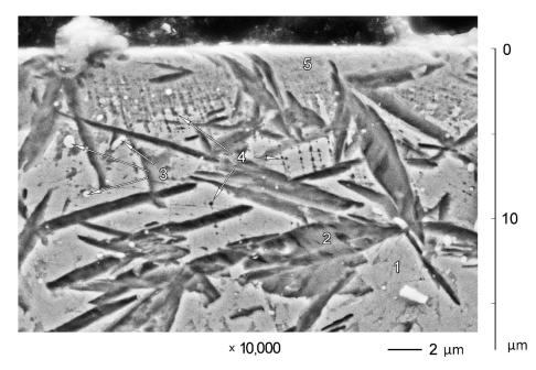
**Figure 4.** Microstructure of subsurface zones of X120Mn3Si2 steel after quenching from 900 °C and wear in A mode: 1—austenite; 2—martensite; 3—carbides; 4—etch pits; 5—surface zone formed by abrasive wear.
