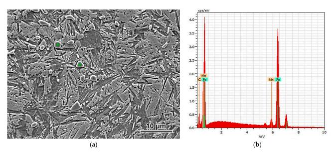
Figure 3. (a) The points of EDX analysis and (b) corresponding EDX spectrum (900 °C-quenched sample).
