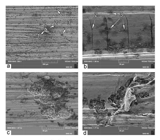
**Figure 8.** SEM micrographs of surface after wear in B mode: (**a**,**b**,**d**) B1000 sample; (**c**) B900 sample; 1—embedded abrasive particle; 2—transverse microcracks; 3—spots of fatigue damage.
