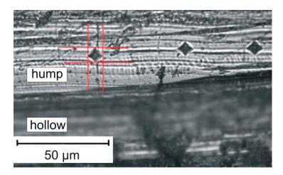
Figure 6. The technique for measuring the microhardness of a worn surface.
