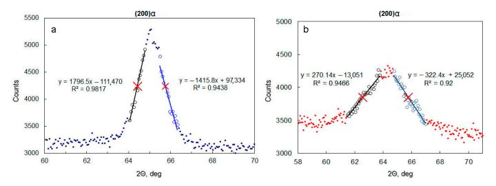
**Figure 1.** Examples of determining Full Width on Half Maximum (FWHM) for  $(200)\alpha$  peak: (a) quenching from 800 °C; (b) B1000.
