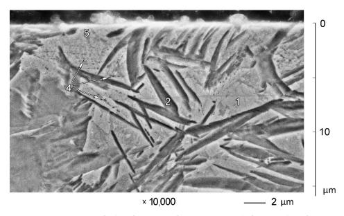
**Figure 5.** Microstructure of subsurface zones of X120Mn3Si2 steel after quenching from 1000 °C and wear in A mode: 1—austenite; 2—martensite; 4—etch pits; 5—surface zone formed by abrasive wear.
