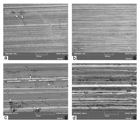
**Figure 9.** SEM micrographs of surface after wear in A mode: (**a**,**c**) A900 sample; (**b**,**d**) A1000 sample: 1—spots of fatigue damage; 2—cracking of ridges.
