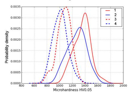
**Figure 7.** Distribution of worn surface microhardness for samples worn in A and B modes: 1—B900; 2—B1000; 3—A900; 4—A1000.
