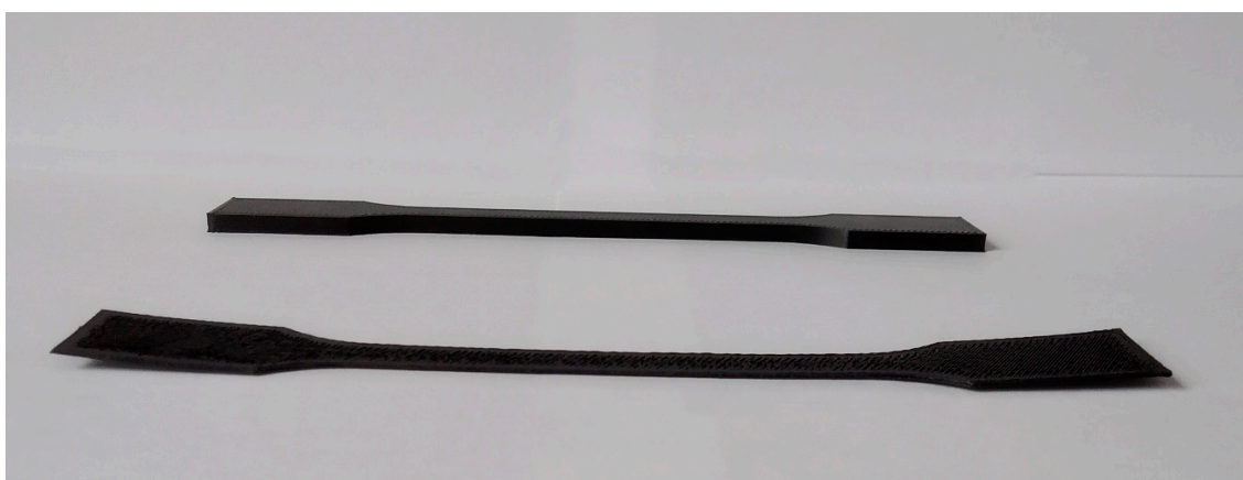
Figure 7. Warping of neat POM at the beginning of the 3D printing compared to the completed specimen.
