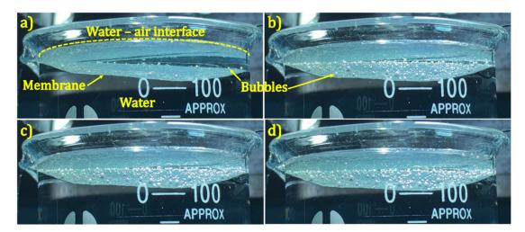
**Figure 4.** Bubbles generated on TiN membrane surface under continuous illumination for (**a**) 30 s, (**b**) 600 s, (**c**) 1200 s and (**d**) 1800 s. The membrane is slightly tilted for better observation.
