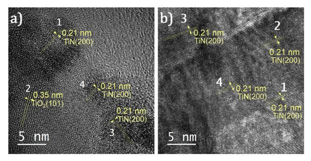
**Figure 2.** HR-TEM images of (**a**) TiON and (**b**) TiN. The lattice spacing was measured using Gatan Micrograph Suite<sup>®</sup> software. The measured lattice spacing of 0.21 nm corresponds to the spacing between (200) planes of TiN, whereas the lattice spacing of 0.35 nm corresponds to the spacing between the (101) planes of anatase TiO<sub>2</sub> [41].
