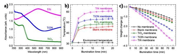
**Figure 3.** (a) UV–VIS absorption spectra of TiO<sub>2</sub>, TiON and TiN nanodonuts, (b) temperature at the surface of membranes under simulated solar light with illuminance of 550 W m<sup>-2</sup>, and (c) the weight change due to water evaporation by different photothermal materials.
