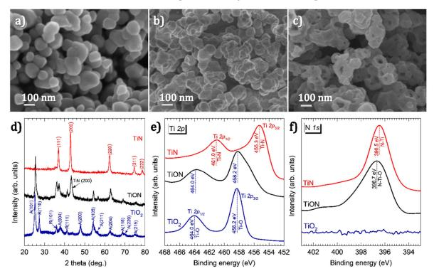
**Figure 1.** SEM images of (**a**) the TiO<sub>2</sub> powder obtained directly from the hydrofluoric acid leaching process and (**b**) after annealing the powder in NH<sub>3</sub> at 700 °C and (**c**) after annealing at 900 °C; (**d**) XRD patterns of the powders in images (**a**–**c**), labelled as TiO<sub>2</sub>, TiON and TiN, respectively; XPS spectra of TiO<sub>2</sub>, TiON and TiN (**e**) at the Ti 2p binding energy and (**f**) at the N 1s binding energy.
