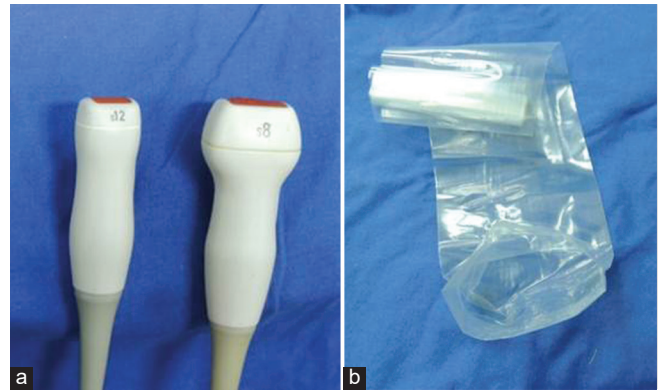
Figure 1: Hardware used for epicardial echocardiography. (a) The probes that are commonly used for the echocardiography generally have the smallest footprint compatible for the patient. In the present case, 12 MHz and 8 MHz frequency that are commonly used in our unit are being displayed. (b) The sterile sheath for the probe
