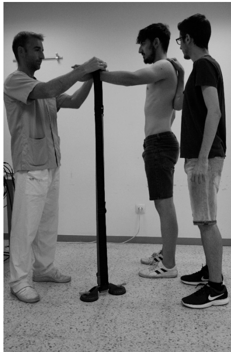
Figure 1. Attachment system for dynamometer measurements.
