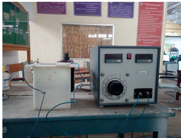
FIGURE 2: Experimental setup of electrowinning process.
