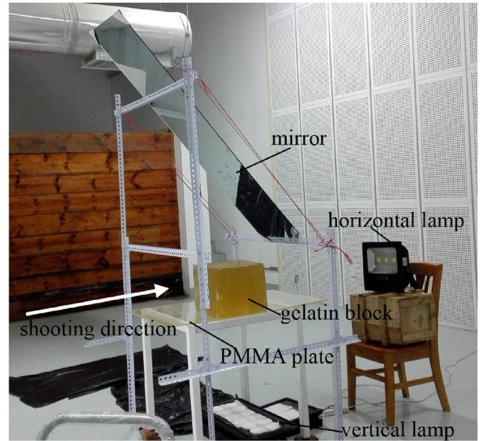
Fig. 1. Placement of the gelatin block. PMMA: polymethyl methacrylate plate.
