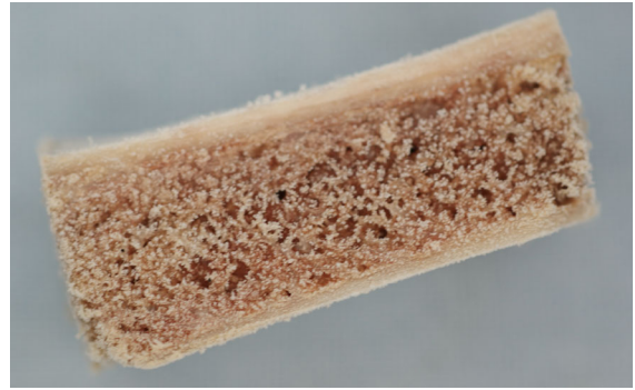
Fig. 3 20 \times 10 \times 10 mm frozen, radiation-sterilised bone block
