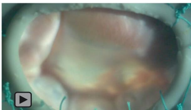
**Video 1:** Acute papillary muscle rupture disease model using the 3D-printed left heart simulator. This specific example of the experimental setup shows a counterclockwise cutting direction (A3?A2) of chordae from the medial head of the posteromedial papillary muscle, starting with 1/3 rupture and incrementally cutting until full rupture is achieved (to see video: <https://youtu.be/jPdFxe5lvlg>).
