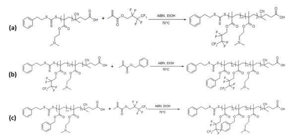
**Scheme 1.** Sequential RAFT alcoholic dispersion polymerization at 70 °C in ethanol using a poly(2-(*N*,*N*,dimethylamino) ethyl methacrylate) as chain transfer agent of: (**a**) heptafluorobutyl methacrylate (HFBMA), (**b**) Benzyl methacrylate (BzMA), (**c**) heptafluorobutyl methacrylate (HFBMA), resulting in the formations of PDMA-PHFBA and PDMA-PHFBMA-PbzMA diblock copolymers ((**a**,**b**) respectively), and PDMA-PHFBMA triblock copolymers (**c**).
