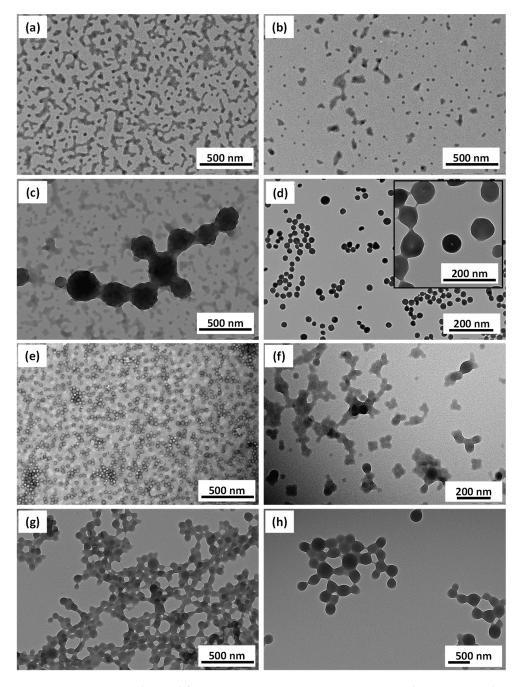
**Figure 4.** TEM images obtained for PDMA<sub>39</sub>–PHFBMA<sub>x</sub>- PBzMA<sub>y</sub> nano objects prepared at 10% w/w with (**a**) x = 50, y = 69; (**b**) x = 99, y = 69; (**c**) x = 149, y = 69; (**d**) x = 199, y = 66; (**e**) x = 50, y = 198; (**f**) x = 99, y = 198; (**g**) x = 149, y = 198; (**h**) x = 199, y = 198.
