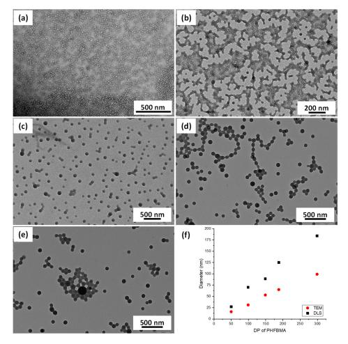
**Figure 3.** TEM images obtained for PDMA<sub>39</sub>–PHFBMA<sub>x</sub> nanoobjects prepared at 10% w/w via RAFT alcoholic dispersion polymerization of HFBMA with (**a**) x = 50, (**b**) x = 99, (**c**) x = 149, (**d**) x = 188, and (**e**) x = 299. (**f**) Evolution of the average particles diameter measured by TEM (red dots) and DLS (black squares) with the DP of the PHFBMA core-forming block.
