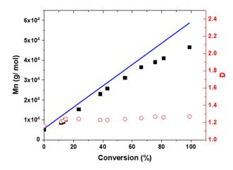
**Figure 2.** Evolution of number-average molar mass ( $M_n$ , black squares) and dispersity (D, red open circles) with conversion for the RAFT dispersion polymerization of HFBMA at 10% w/w solids in ethanol at 70 °C using a PDMA<sub>39</sub> macro-CTA with macro-CTA/AIBN molar ratio of 5/1. The targeted diblock composition was PDMA<sub>39</sub>–PHFBMA<sub>200</sub>.
