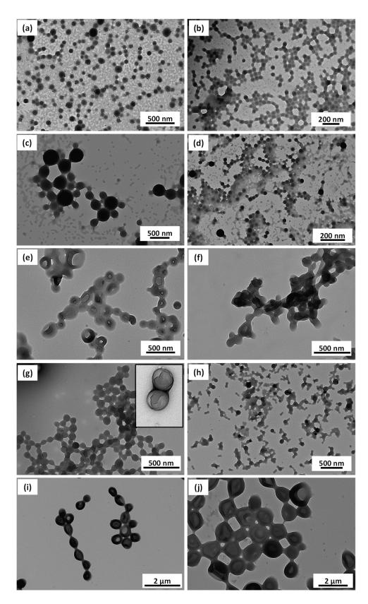
**Figure 5.** TEM images obtained for PDMA<sub>39</sub>-PBzMA<sub>x</sub>-PHFBMA<sub>y</sub> nano objects prepared at 10% w/w with (**a**) x = 69, y = 50 (**b**) x = 69, y = 99 (**c**) x = 69, y = 149 (**d**) x = 69, y = 196 (**e**) x = 99, y = 65 (**f**) x = 149, y = 141 (**g**) x = 198, y = 50 (**h**) x = 198, y = 96 (**i**) x = 198, y = 144 (**j**) x = 198, y = 189.
