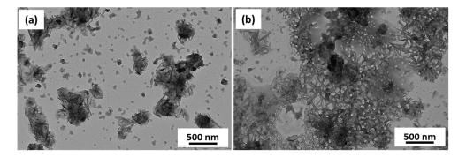
**Figure 6.** TEM images obtained for PDMA<sub>58</sub>–PBzMA<sub>198</sub>-PHCFDDMA<sub>x</sub> prepared at 10% w/w with (**a**) x = 19 (**b**) x = 50.
