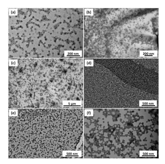
**Figure 7.** TEM images obtained for PDMA<sub>58</sub>-PBzMA<sub>x</sub>-PTDFOA<sub>y</sub> self-assembled nano objects prepared at 10% w/w by RAFT dispersion polymerization of PTDFOA in ethanol, with (**a**) x = 69, y = 48 (**b**) x = 69, y = 91 (**c**) x = 69, y = 144 (**d**) x = 194, y = 44 (**e**) x = 194, y = 83 (**f**) x = 194, y = 120.
