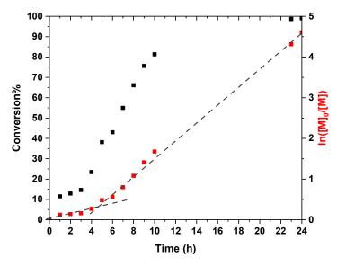
**Figure 1.** Kinetic data (Conversion %: Black squares, Semi-log: Red squares) obtained for the RAFT dispersion polymerization of HFBMA at 10% w/w solids in ethanol at 70 °C using a PDMA<sub>39</sub> macro-CTA at a macro-CTA/AIBN molar ratio of 5/1. The targeted diblock composition was PDMA<sub>39</sub>–PHFBMA<sub>200</sub>.
