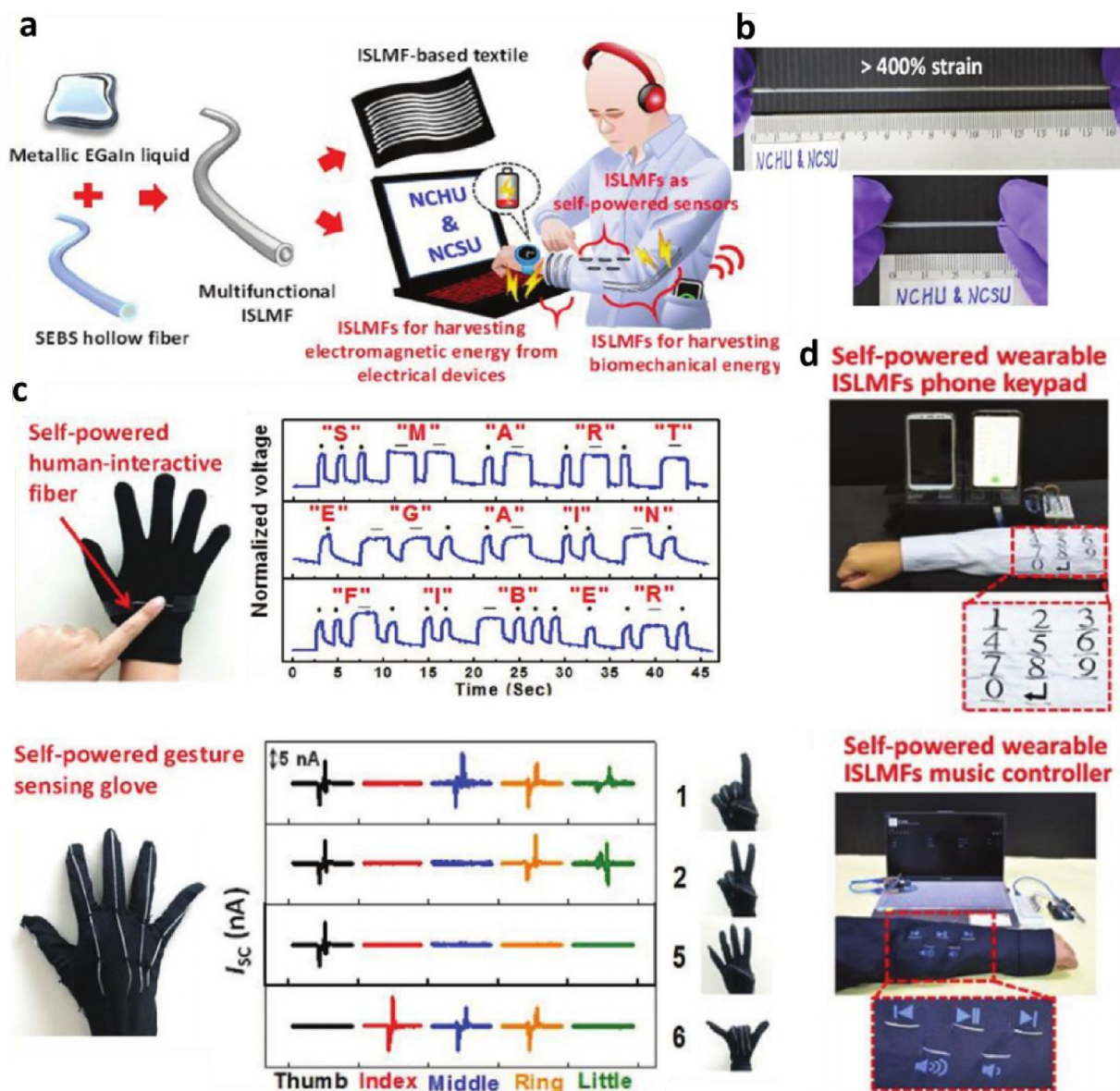
Figure 6. Advanced materials for textile-based wearable electronics. (a) Fabrication of liquid-metal fiber based TENG for energy harvesting and self-powered sensing. (b) Illustration of the ultrastretchability of the fiber. (c) Application of the fiber as a self-powered human-interactive fiber and gesture glove. (d) Application of the fiber as a wearable keypad and music controller. Reproduced with permission from ref 120. Copyright 2021 John Wiley and Sons.
