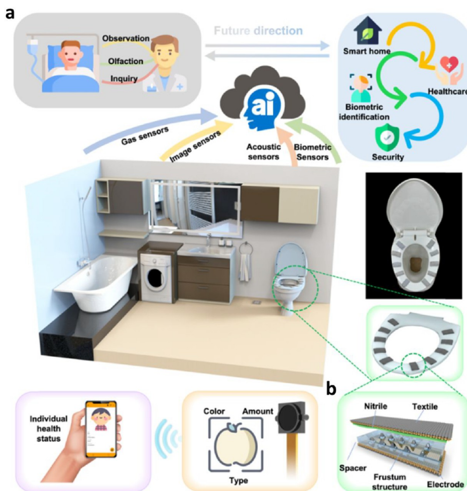
Figure 42. AI-Toilet by fusing the triboelectric and image sensing technology. (a) Schematic of the AIoT enabled toilet for health monitoring. (b) Detailed structure of the TENG sensor. Reproduced with permission from ref 248. Copyright 2021 Elsevier.
