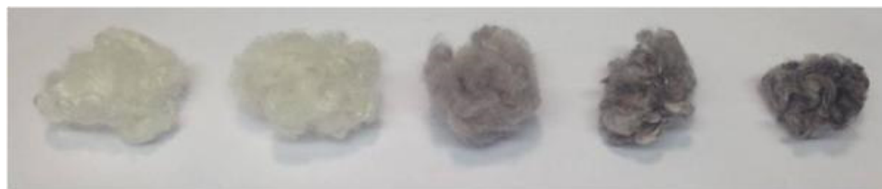
Figure 8. Photograph of impregnated silks, from left to right : native silk, control impregnation (no \text{scCO}_2 ), \text{scCO}_2 impregnation 0.1, 0.3, and 0.6 O.D, respectively.
