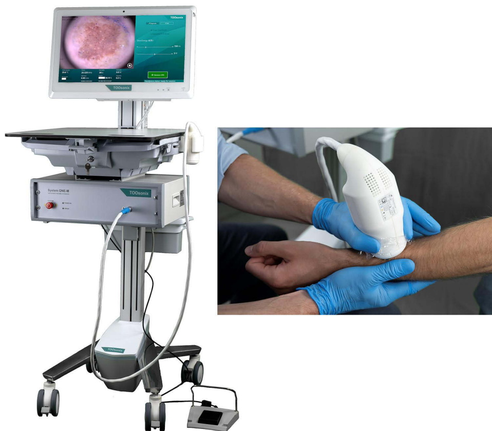
Figure 3 TOOsonix HIFU system operating at 20 MHz. The handpieces have an integrated real-time video camera allowing accurate control and monitoring of the treatment.
