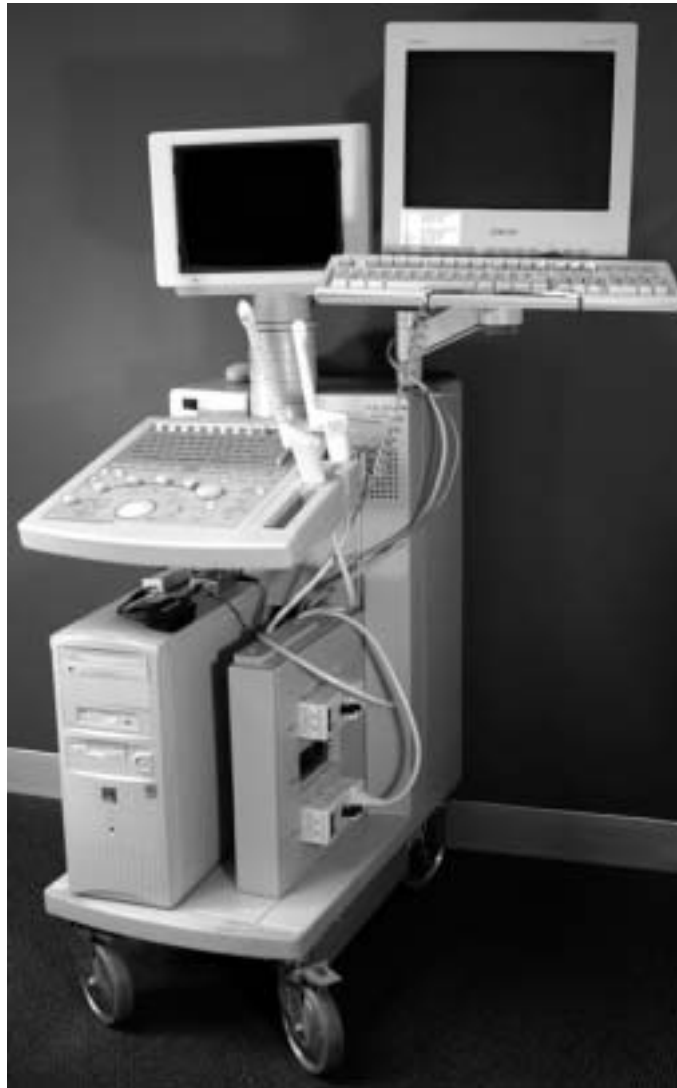
Fig. 1. Clinical scanner configured for data acquisition. A Hitachi EUB 525 instrument provides RF data to the PC computer system on its lower shelf (in the lower left corner of the figure). The keyboard and larger monitor (in the upper right corner of the figure) provide the user interface for the data-acquisition computer. RF signals are acquired from the scanner after summation of the individual array-element signals but prior to non-linear amplification or other processing.
