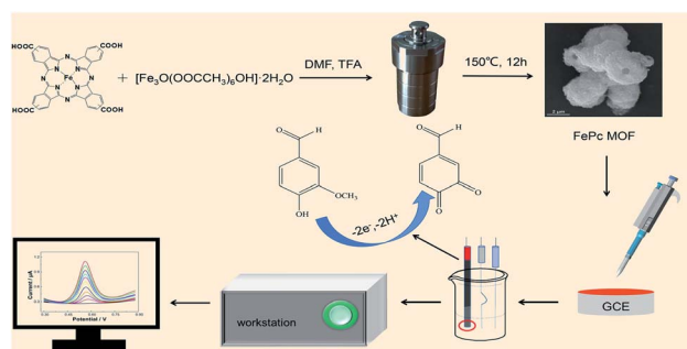
Scheme 1 Fabrication of FePc MOF/GCE modified electrode and electrochemical determination of vanillin.
