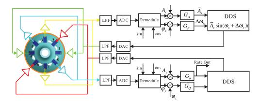
For the circuit system's hardware application, the control loops and DDS signals are generated from DSP. The signal collecting is done by DAC. The piezoelectric electrodes' driving and detecting use the analog conditioning circuit. In the real circuit system, we use the STM32F405 as the DSP chip, DSP to supply ADCand AD5328 as the DAC chip. The core component of the analog conditioning circuit is AD8676.
