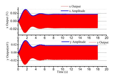
Figure 17. The gyro's output with control in  $\Omega = 0$ .
