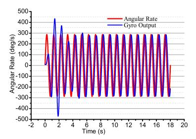
**Figure 23.** The calculated angular rate output with control in  $\Omega$  is square.
