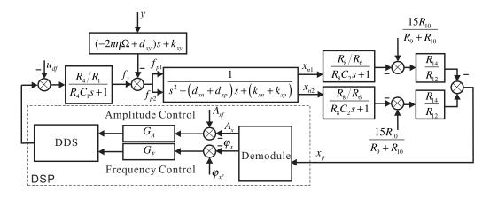
Figure 13. The structure frame of the *x*-axis control loop.
