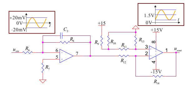
In the detecting components, firstly, the signal should pass a filter amplifying process to remove the high frequency vibratory noise, and then, it should be adjusted to meet the requirement for the ADC to sample. To meet the requirement of signal conditioning, we choose  $\frac{R_{14}}{R_{12}} = \frac{R_{13}}{R_{11}}$ ; the relation between inputs and outputs for a circuit in low-pass filter's pass-band is:
