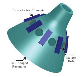
Figure 1. The schematic of the bell-shaped resonator's structure.
