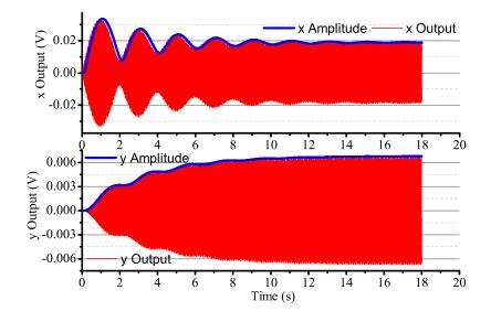
**Figure 16.** The gyro's output with non-control in  $\Omega = 0$ .
