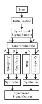
After initialing the system, DSP samples the ADC synchronously, collects the signals of the x-axis (piezoelectric Electrodes 3 and 7) and the y-axis (piezoelectric Electrodes 4 and 8), goes through linear
