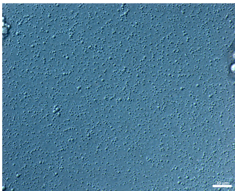
Figure 5. Optical microscopy (Magnification 20x) of BC emulsions with o/w 20/80 prepared with 1 wt % CAS while using sonication. Scale bar is 10 \mu\text{m} .
