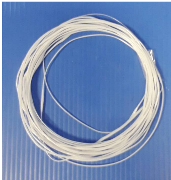
Figure 6. PLA filaments fabricated by recycling material addition ratio of 60%.
