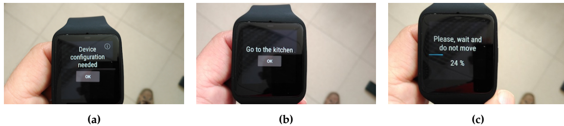
Figure 6. Some procedure steps to map the environment and create the Machine Learning classifiers. (a) Configuration starting; (b) User asked to go to the kitchen; (c) Sampling WiFi signal strength.
