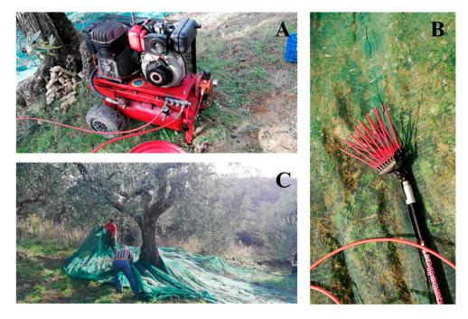
**Figure 6.** (**A**) Air compressor with 5.5 kW diesel engine; (**B**) pneumatic combs for olive harvesting; (**C**) laying nets for the interception of olives on the ground.
