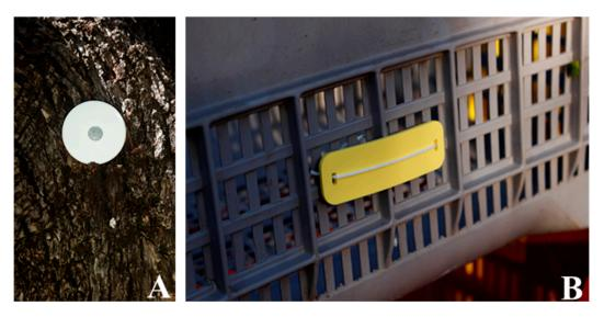
**Figure 2.** (**A**) The RFID1 standard used is UHF at 860 MHz, Class 1 Gen 2, waterproof coin shaped with central hole; (**B**) the RFID2 is UHF at 860 MHz, waterproof flexible band with two holes at the extremities fixed with a small cord on the crate.
