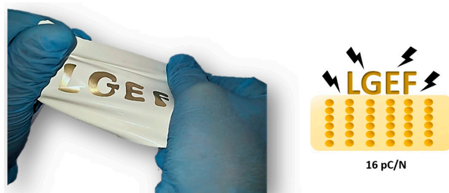
Figure 9. Picture of stretched piezoelectric sensor developed in this study.
