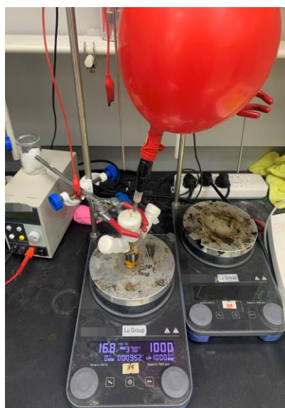
Supplementary Figure 12. The reaction mixture was electrolyzed at a constant current of 4 mA and irradiated with a 20 W purple LED lamp (0.5 cm away, with cooling fan to keep the reaction temperature at 25 °C) for 12 h.
