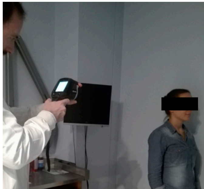
Figure 5. Recording the right lateral thermograms with the thermal imaging infrared camera, E60 FLIR.
