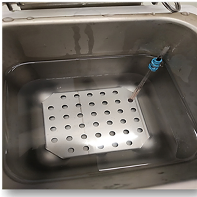
Fig. 5. Capillaries placed together in a water bath for amplification at 65 °C.
