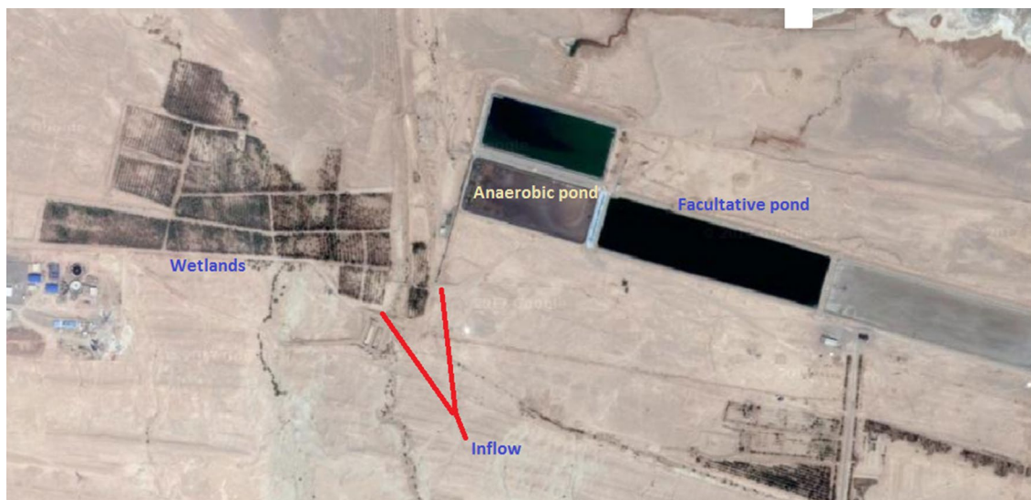
Fig. 1 The position of wastewater stabilized ponds (WSPs) and artificial wetlands of Yazd wastewater treatment plant
