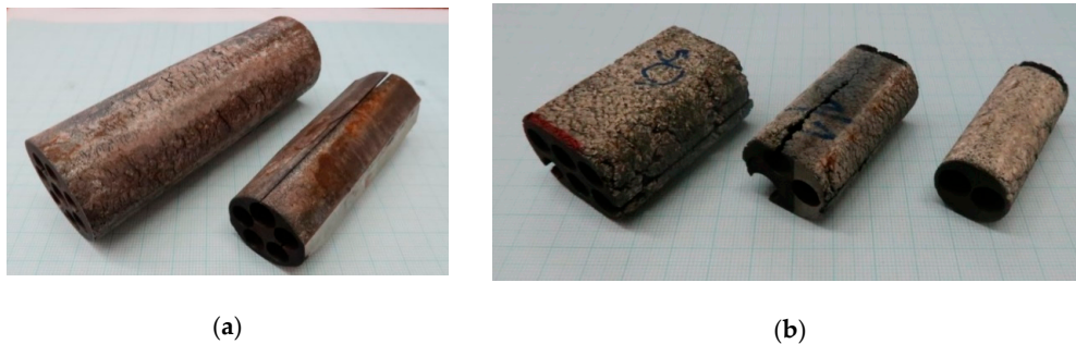
Figure 1. Photographs of (a) forged rods and (b) rolled rods. The samples for tensile and fatigue testing were already machined from the processed conditions parallel to the axial direction. SEM samples were prepared from cross-section of rods.
