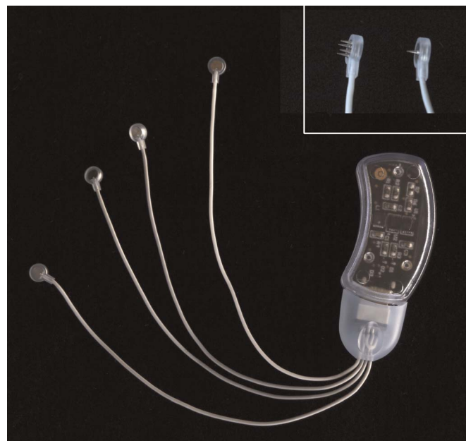
Figure 2. A percutaneous auricular nerve stimulation system (NSS-2 Bridge; Masimo, Irvine, CA). Each of the three electrodes has a 2-mm-long integrated needle/lead (inset) and the ground electrode has four 2-mm-long integrated needles/leads (inset). Used with permission from Brian M. Ilfeld, MD, MS.
