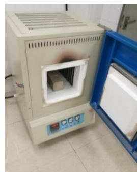
Figure 5. Muffle furnace with the function of programming control.
