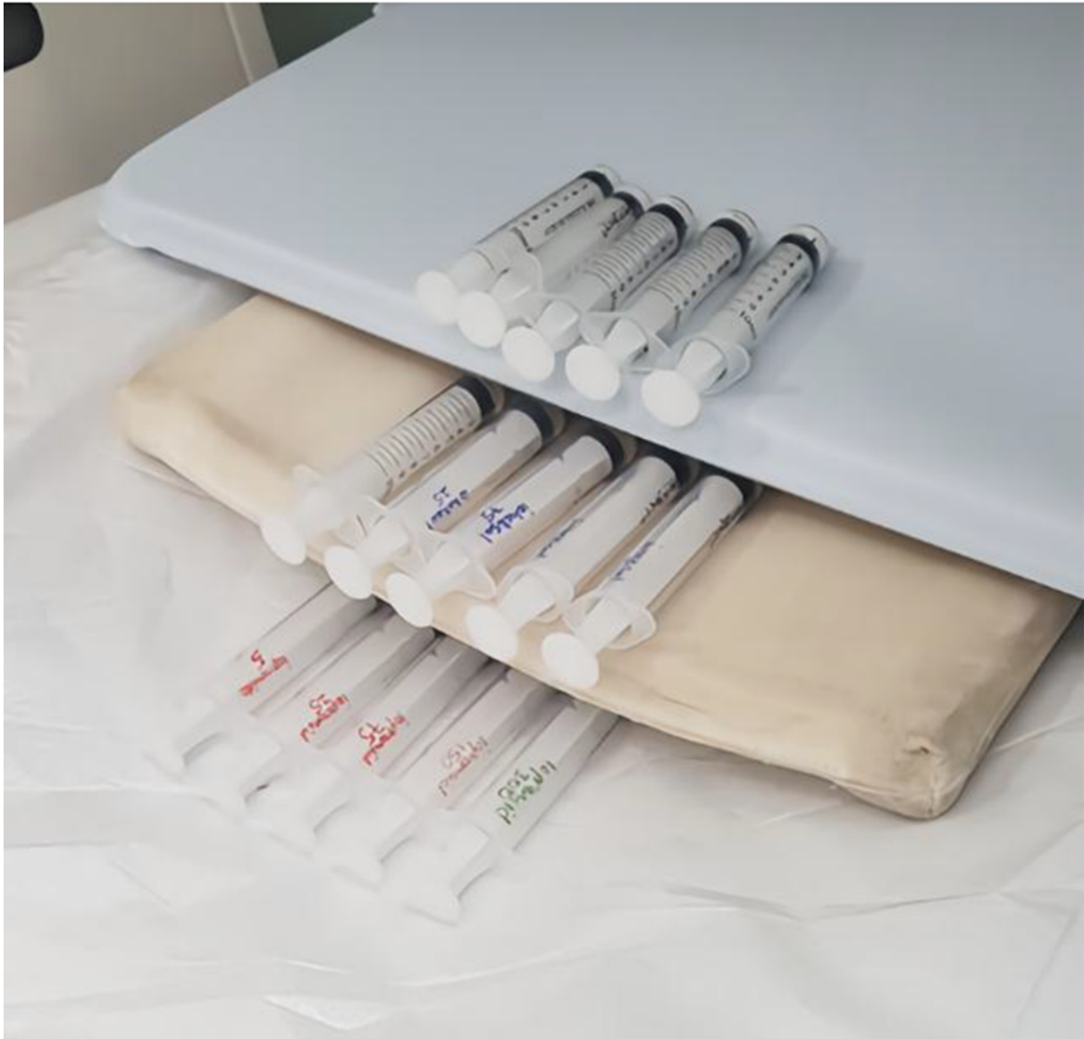
Figure 3. The samples (upper line 4N-TIB nanosuspension, middle line iohexol, bottom line iopromide) are in the gantry of CT.
