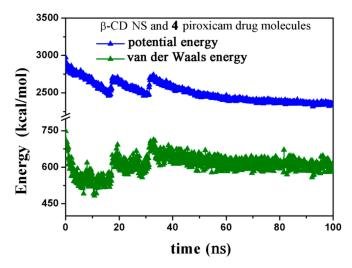
**Figure 6.** The potential energy and the van der Waals contribution calculated during the MD run for the NS model interacting with 4 piroxicam molecules.
