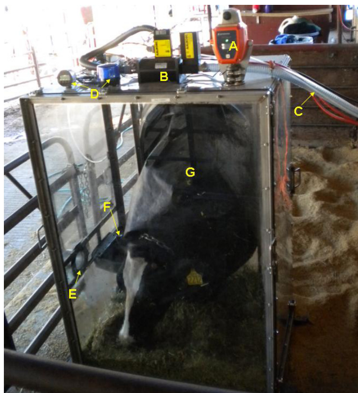
Figure 4. A dairy cow standing and eating during a gas sampling period. (A) is the oxygen sensor/alarm; (B) is the mass flow controller; (C) is the main air line that was connected to the rotary vane vacuum pump; (D) is the differential pressure gage/alarm system; (E) is the air inlet opening; (F) is the water bowl for the cow; (G) is the neck sleeve.
