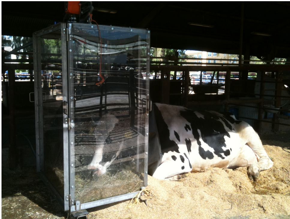
Figure 4. A dairy cow standing and eating during a gas sampling period. (A) is the oxygen sensor/alarm; (B) is the mass flow controller; (C) is the main air line that was connected to the rotary vane vacuum pump; (D) is the differential pressure gage/alarm system; (E) is the air inlet opening; (F) is the water bowl for the cow; (G) is the neck sleeve.
