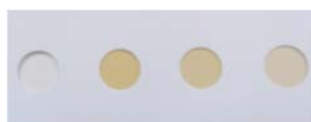
Figure 3. Silica gel supported probes in presence of increasing amounts of formaldehyde gas for 30 min (from left to right 0, 40, 16 and 8 ppm of formaldehyde).
