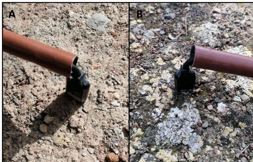
Fig. 3 Pictures of the EC-5 moisture sensors used in open areas devoid of perennial vegetation with very low (<5%, A ) and high (>75%, B ) cover of biocrust-forming lichens.
