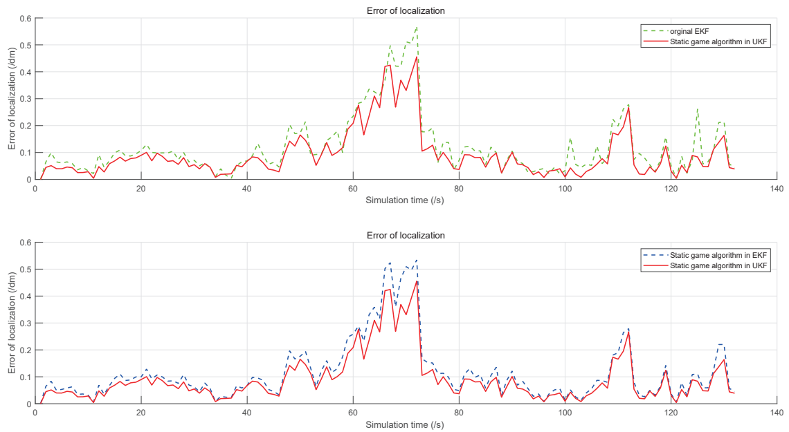
Figure 8. The error of localization on the game theory UKF, the original extended Kalman filtering (EKF), and the game theory EKF.
