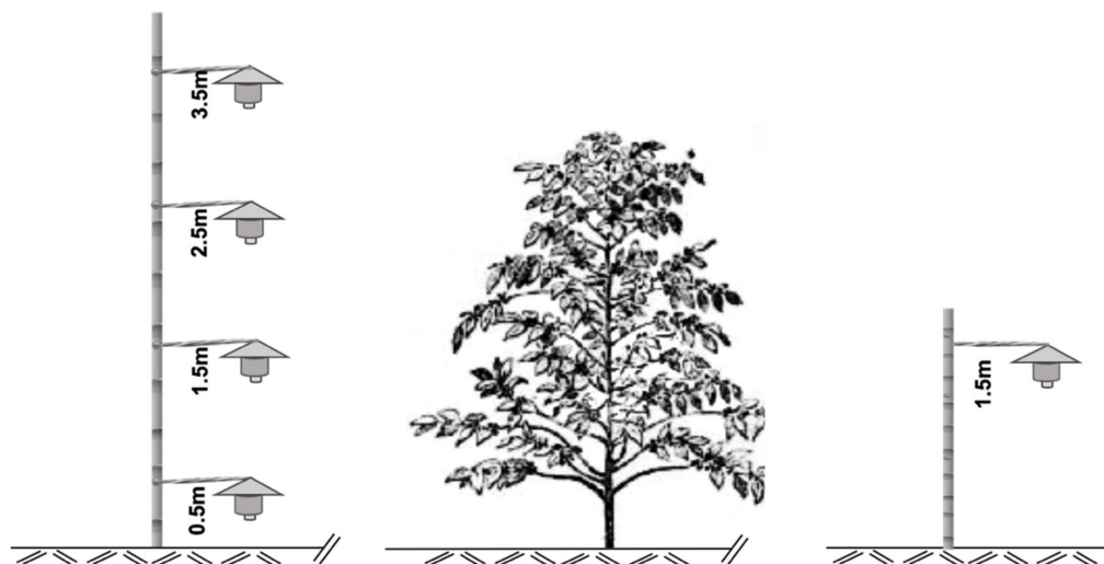
Figure 1. Representative illustration of column traps (CT). Each CT comprised of four traps placed at 0.5 m, 1.5 m, 2.5 m, and 3.5 m above ground and a single trap (ST) at 1.5 m above ground. The field experiments were conducted in Adjuntas, Puerto Rico.
