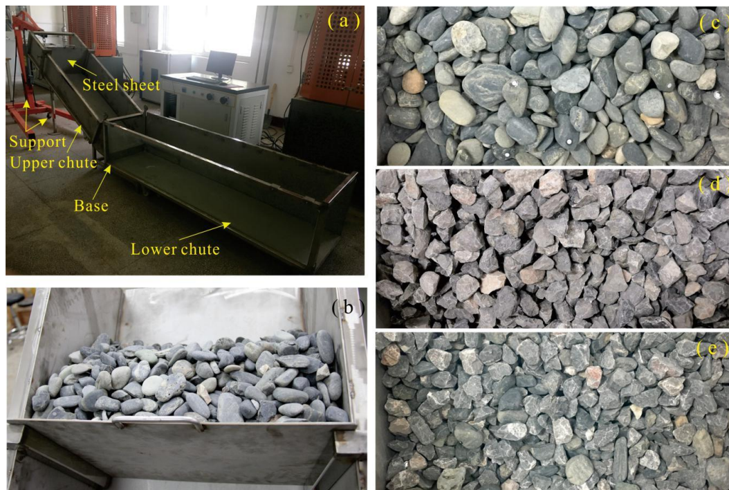
Figure 1. The experiment equipment and sliding materials used in physical model: (a) flume, (b) steel sheet, (c) pebbles, (d) gravels, and (e) mixtures.
