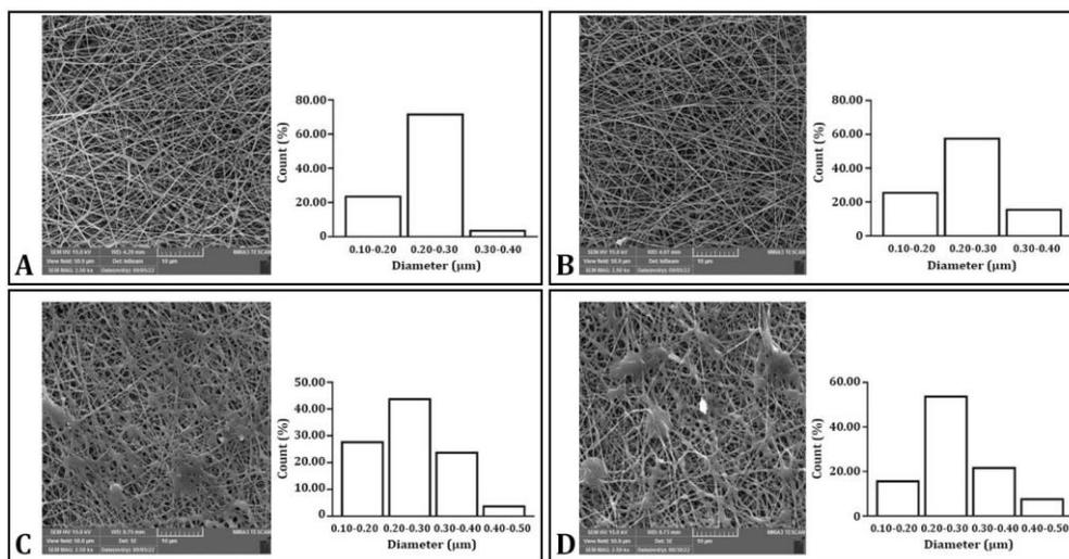
**Fig. 1.** Field emission scanning electron microscopy images of the synthesized **A)** Polycaprolactone (PCL)/Curcumin (Cur), **B)** PCL, **C)** PCL/Vancomycin (Van), and **D)** PCL/Cur/Van nanocomposites.
