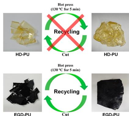
**Figure 9.** Recyclable capacity of EGD-PU with a hot press (photograph courtesy of Se-Ra Shin. Copyright 2021).
