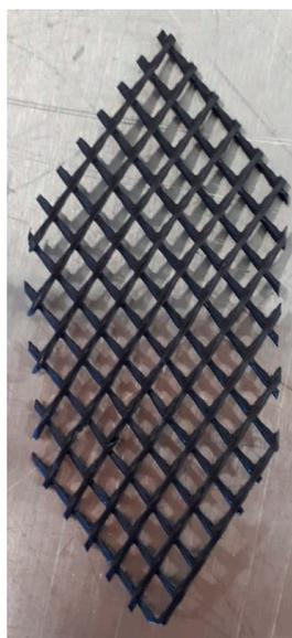
**Figure 2.** Photograph of the spacer used inside the ED channels.
