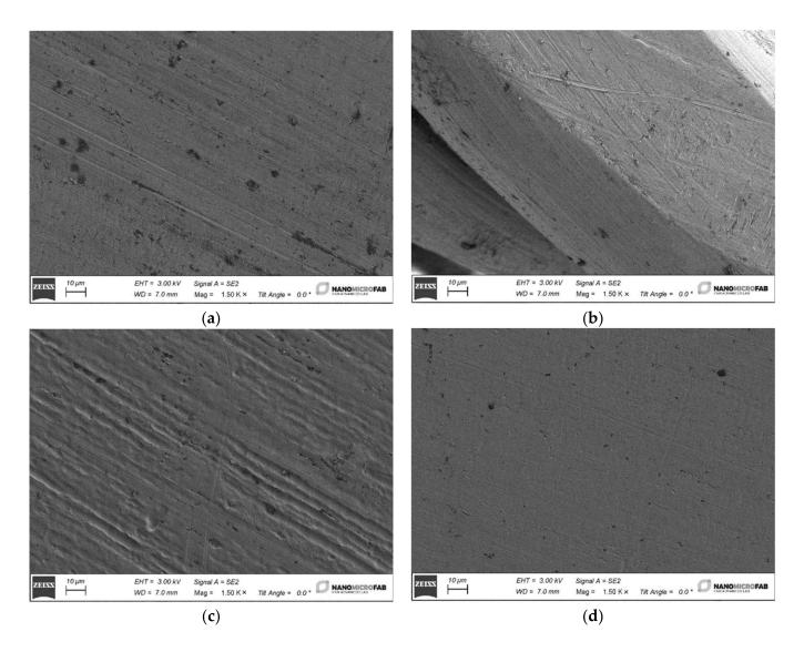
**Figure 3.** Four SEM images of the different "as is" samples at a magnification of 1500×: (**a**) SS AISI 304 Extra-hard; (**b**) SS AISI 302 Twist; (**c**) Ni–Ti; (**d**) SS AISI 304 S.
