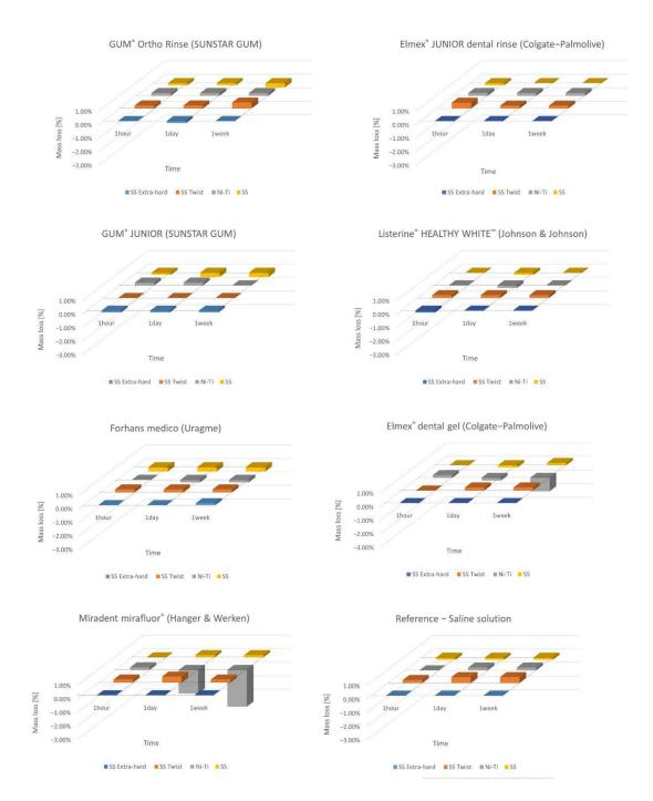
**Figure 1.** Differences in weight percentage of the 96 orthodontic arch section samples (n = 24) after 1 h ( $t_1$ ), 24 h ( $t_2$ ) and 168 h ( $t_3$ ) of storage in the different fluorinated agents. One-way ANOVA for each individual substance in which the four different orthodontic alloys were immersed for three different time intervals has been performed. The weighted average of the five weighings was calculated and finally the relative difference from the initial weight was obtained.
