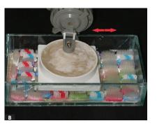
Figure 9 - A) Teeth attached to a sink strainer so as to form a single specimen to be taken to the brushing machine; B) Brushing machine comprised by a glass box with tooth brush heads attached to the bottom with hot glue. The engine of a security camera was adapted to perform round-tripping movements.
