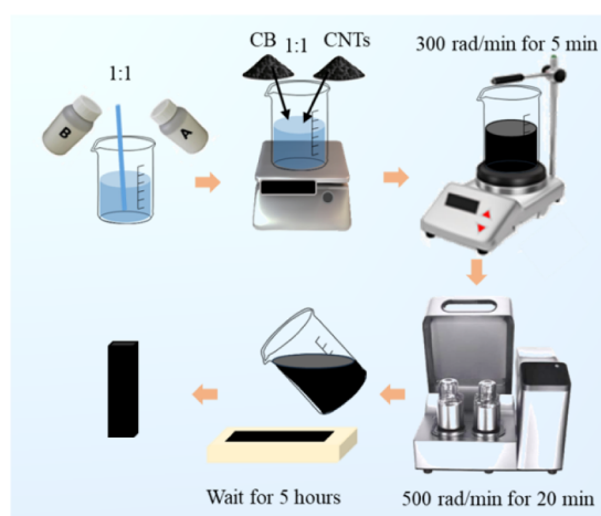
Figure 1. Resistance–strain sensor prepared by a mechanical mixing method.
