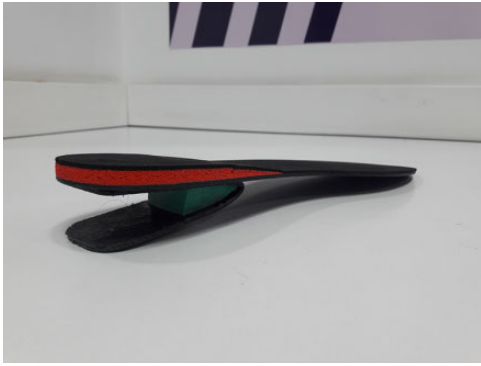
Figure 1. Propulsion heel-lift orthotic. A flexible spring of polycarbonate (bent black piece) was placed under the rear side of the polypropylene flat layer of 3 mm (black fiber). Red low-hardness ethylene-vinyl-acetate (EVA) was used to cushion the polycarbonate junction with polypropylene on the upper layer, and green medium-hardness EVA was used to cushion the angular corner of the spring.
