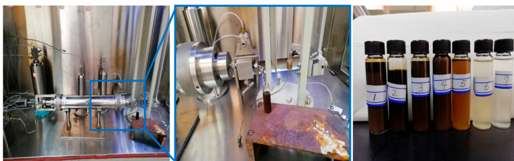
Figure 10. Core flooding experimental apparatus (left); The fluids produced at different times during the surfactant flooding process were collected (center); Starting from the first drop of oil at the outlet, samples #1–#7 were collected at regular intervals of 10 min (right).
