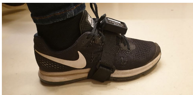
Fig. 1 Positioning of the inertial measurement units
