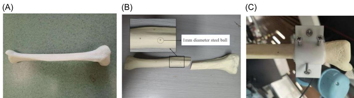
**FIGURE 14** Model bone. (A) Tibia model bone. (B) Model bone after amputation. (C) Distal bone jig and fixation.
